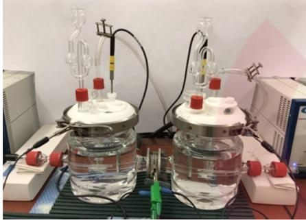
Hydrogen Electrochemical Permeation Tests
