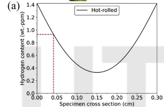
$$C_{tot} = \frac{C_0}{r} \left( \operatorname{erfc}\left(\frac{x}{\bar{x}}\right) - \frac{\bar{x}}{\sqrt{\pi}} e^{-\left(\frac{x}{\bar{x}}\right)^2} + \frac{\bar{x}}{\sqrt{\pi}} \right) \text{ where } \bar{x} = 2\sqrt{D_{eff}t}$$
