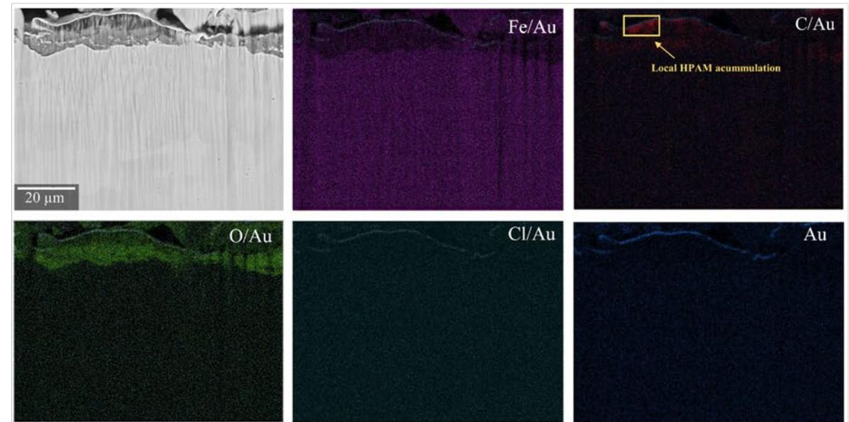
CO<sub>2</sub>-saturated + 1.5 wt. % NaCl + 1000 ppm HPAM
