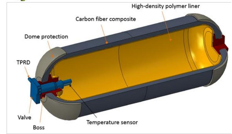
Design of hydrogen storage tanks under fatigue and vibration condition
