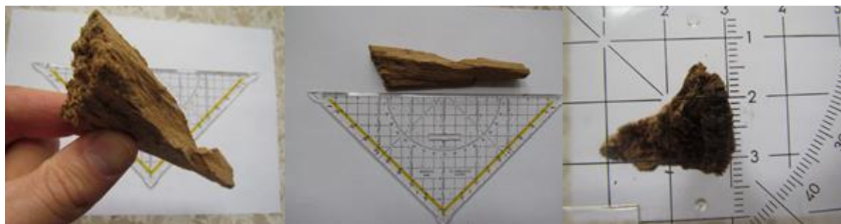
Figure 3. Measuring the cross section area of the largest particle using a set square. The measurement result is around 2.25 \text{ cm}^2 . Photos: Holzforschung Austria.
